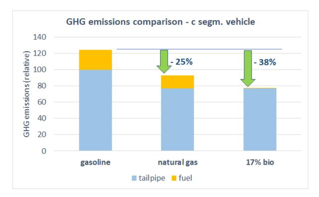
This effect is even of more interest as it is performs under every operating conditions of the engine. Being related to the fuel characteristics, this is key to guarantee the same value of  $CO_2$  reduction independently from the driving conditions, from the load of the vehicle or the ambient temperature.
